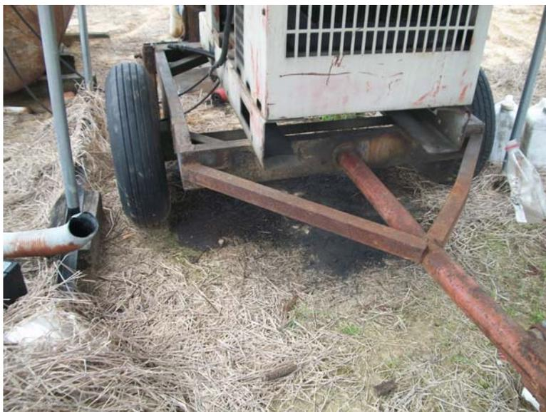
Oil staining below diesel engine.
