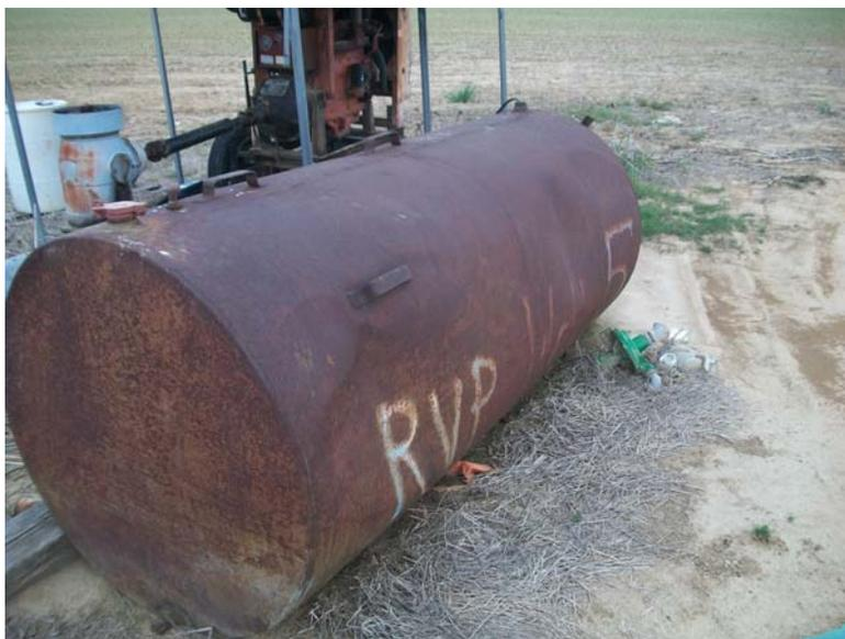
Dent and corrosion on Tank No.2.
